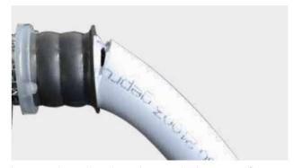
Flexible springs or benders are approved as auxiliary tools. When bending with the inner flexible spring, the pipe end must firstly be deburred. During the bending procedure, the ribs of the flexible spring may not be visible on the outer coating.
