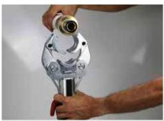
Open the press jaws by pushing the axle strub between thump and index finger.
